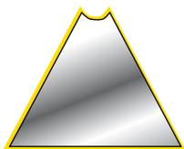
Pre-tap hole size is correct. Thread percentage is 65-75%, and the after-tap minor diameter is in specification.
